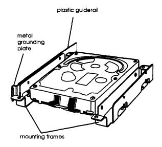
2. Then remove the two screws securing each mounting frame to the drive and remove the frames.
